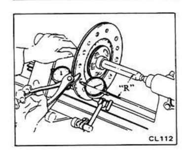
5. Check fit of disc hub on transmission main drive gear splines for smooth sliding. If splines are worn, clutch disc or main drive gear should be replaced; that is, backlash exceeds the specified value at outer edge of clutch disc.
