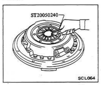
Also, unevenness of diaphragm spring toe height should be within the specified limit.
