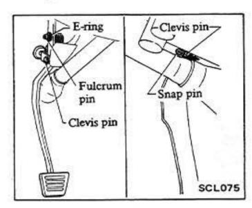
After removing E-ring (160 series) or bolts and pedal shaft plates (61 series), remove or pull out fulcrum pin, then remove clutch pedal and return spring.
