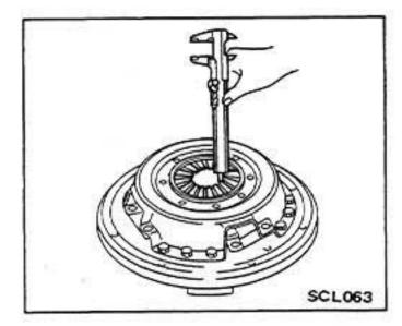
If height "A" of spring end is beyond specified value, adjust spring height with Tool ST20050240. If necessary, replace clutch cover assembly.
