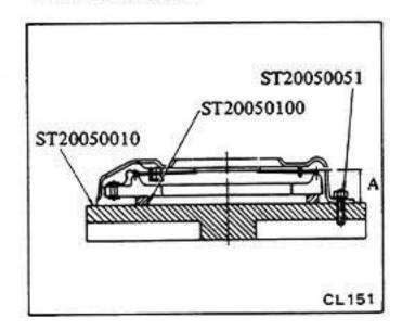
(2) Measure height "A" at several points with a vernier caliper depth gauge.
