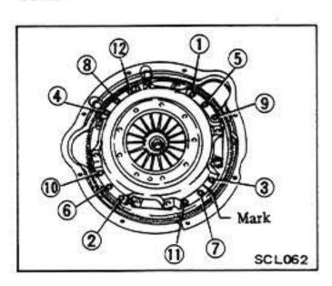
Remove clutch disc and cover assembly.
