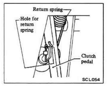
After assembly, adjust clutch pedal height and free play. Refer to Clutch Pedal Height and Free play (Section MA):
