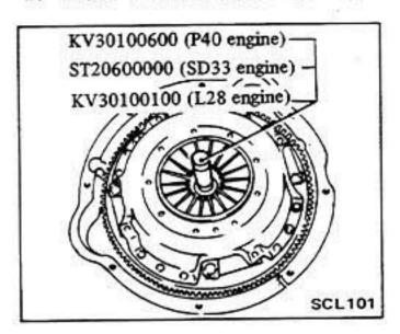
Loosen bolts attaching clutch cover to flywheel, one turn each at a time, until spring pressure is released.
