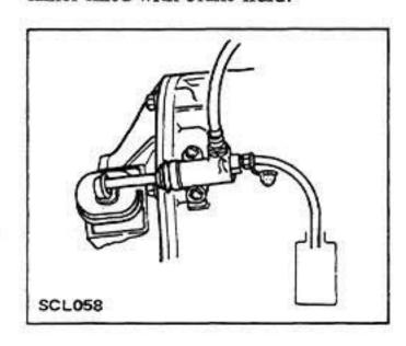
Have a co-worker depress clutch pedal two or three times. With clutch pedal depressed fully, loosen bleeder screw to bleed air out of clutch system.
