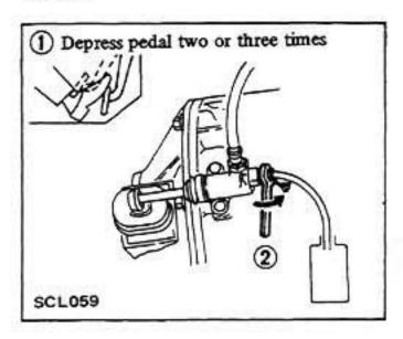
Close bleeder screw quickly as clutch pedal is on down stroke.
