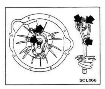
A small amount of grease should be coated to the above points. If too much lubricant is applied, it will run out on the friction plates when hot, resulting in damaged clutch disc facings.
