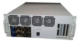
Open Connect Appliances are servers based on commodity PC components (similar to the model used by all large scale content delivery networks). We were influenced by the excellent write-ups from the Backblaze team, and use a custom chassis due to a lack of ready made options for a compact unit.
